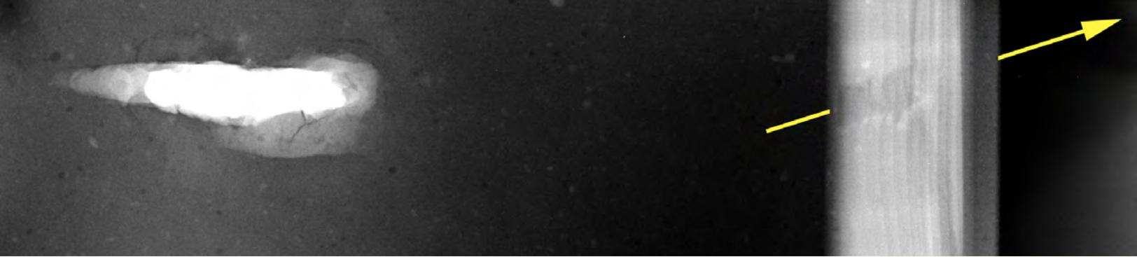
▲ **Figure 11: X-ray image of acutely impacting bullet hole in drywall and 2x4 board. An upward deflection is evident from the perforation of the board (front view).**
