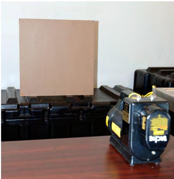
◀ **Figure 4: X-ray set-up showing x-ray source in foreground and test wall 1 with patched bullet holes in background.**
