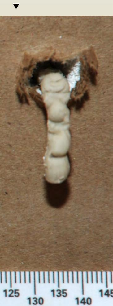
During this process, putty was extruded through the back of the hole and a ragged cylinder of putty hung from the back of the hole (figure 6). These fell off when the wall was moved for x-ray, but may still be present on an actual wall repaired in this fashion.
