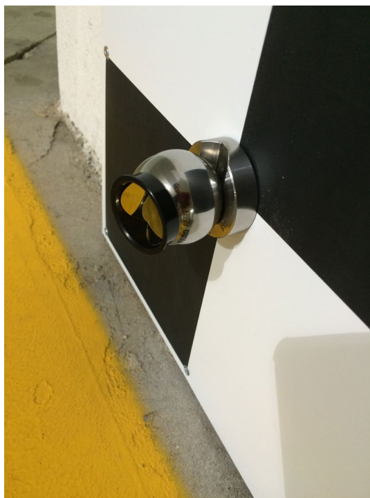
FIGURE 1: Sample checkerboard target. Note the laser tracker SMR inserted into a center hole, which provided a discrete location for the laser tracker to measure.
